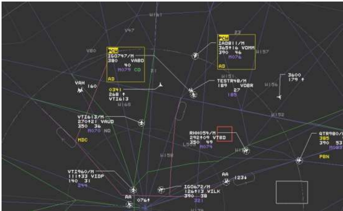
Figure: At 05:53:10 UTC, Predicted Conflict Warning got generated on Automation System.
